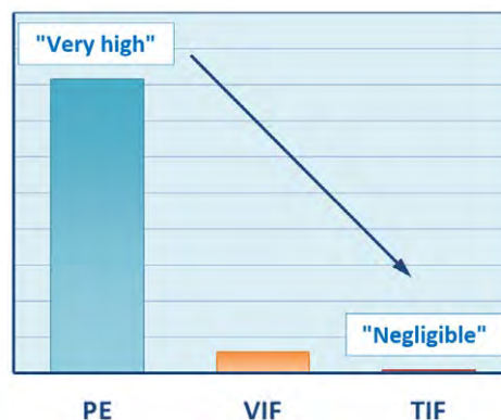
Relative permeability of fumigant gases through polyethylene (PE), virtually impermeable film (VIF) and totally impermeable film (TIF)
